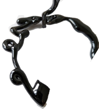
▲ Molten and resolidified regolith simulant (manual pouring experiments)
