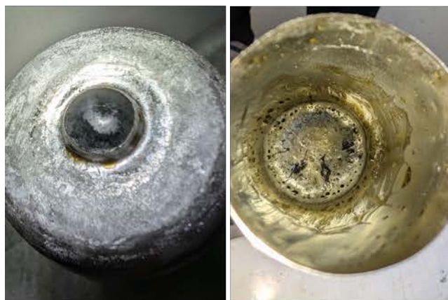
Crucible after outflow: ~6 g remain in crucible
