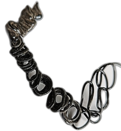
▲ Molten and resolidified regolith simulant (manual pouring experiments)
